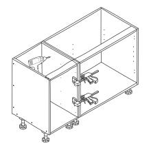
Attach the cabinets together using using 28mm wood screws (h).
