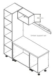
This slimline cabinet can be used in conjuction with pantry end panels as an overhead refrigerator cabinet.
