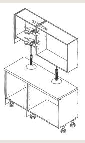
Check again that all of your cabinets are level. If you have a plasterboard wall, attach cabinets using timber screws that are at least 65mm in length. Ensure each screw is inserted through a timber stud.
